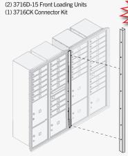
4C horizontal mailbox connector kits connect recessed mounted units side by side and eliminate the need for wood
