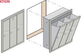
Note: For U.S.P.S. accessed vertical mailboxes, the master lock in the top tier of mailboxes must be no more than 58" above the finished floor. The master lock in the bottom tier of mailboxes must be no less than 30" above the finished floor. No more than two (2) tiers of mailboxes may be installed.
