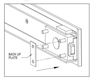
Step 6 Install and tighten the six (6) lock nuts onto the six (6) captive bolts. **DO NOT OVERTIGHTEN THE NUTS.**
