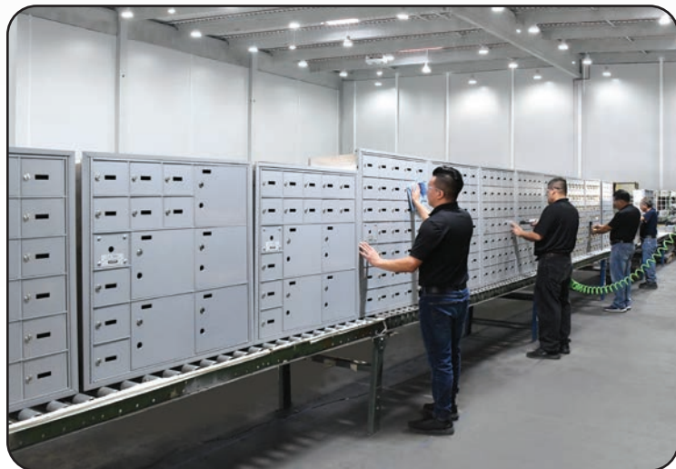
Final inspection of custom horizontal units
