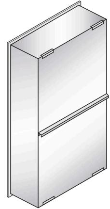
Rear loading unit with non-locking, removable lift off rear cover displayed
