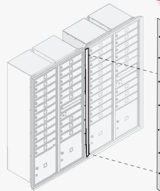
4C horizontal mailbox connector kits connect recessed mounted units side by side and eliminate the need for wood studs between the units.
