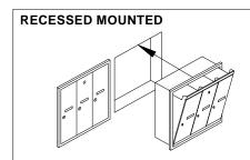
Units fit into a rough opening and are secured with mounting hardware through the back or side panels of the unit.
