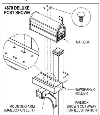
Note: On the 4870 deluxe mailbox post, the longer mounting arm which accommodates the newspaper holder and mailbox can be on either the left or right side. When attaching the post to the ground, position the post so the longer mounting arm is on the side desired. Then mount the newspaper holder and mailbox on the mounting arm with the mailbox facing the street or roadway.
