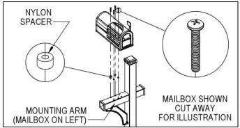
Note: On the 4870 deluxe mailbox post, the longer mounting arm which accommodates the mailbox can be on either the left or right side. When attaching the post to the ground, position the post so the longer mounting arm is on the side desired. Then mount the mailbox on the mounting arm with the mailbox facing the street or roadway.
