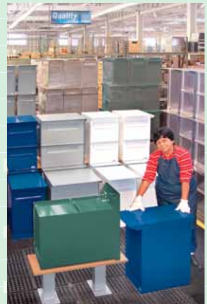
Final inspection of pedestal drop boxes
